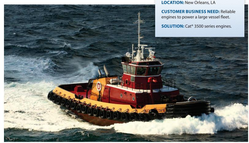
are the 3500 series, and most of them are Cat 3516C engines. We do run 2 vessels with 3512Cs and one that has 3516Bs. We also have a tug that's still nicely running its D399s." In 2007, the company built their first Z drive tractor tug, powered by the 3516C engines and have grown their relationship with Louisiana Cat and Parts Sales & Service Representative, Michael Murzi, over the past several years.
