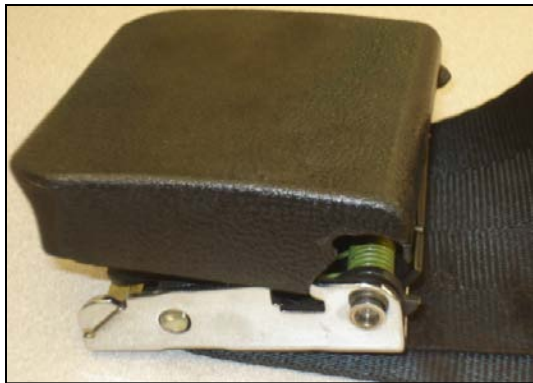
Visible damage to non-retractable buckle
