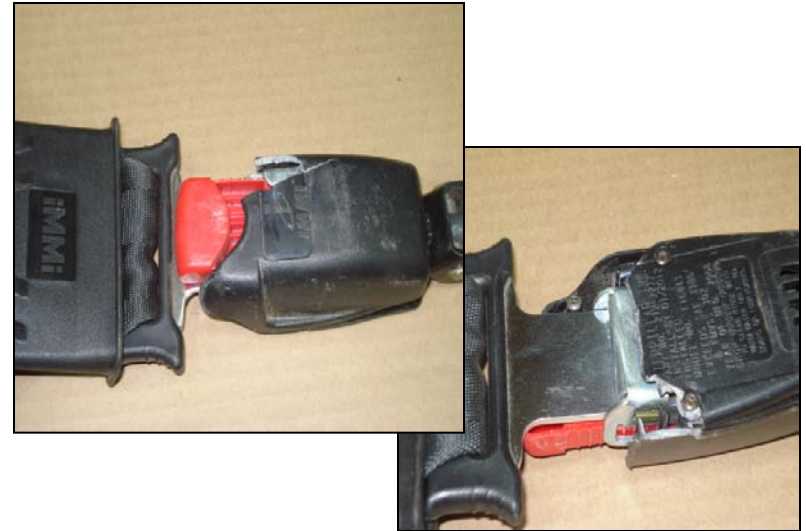
Damage due to force / impact
