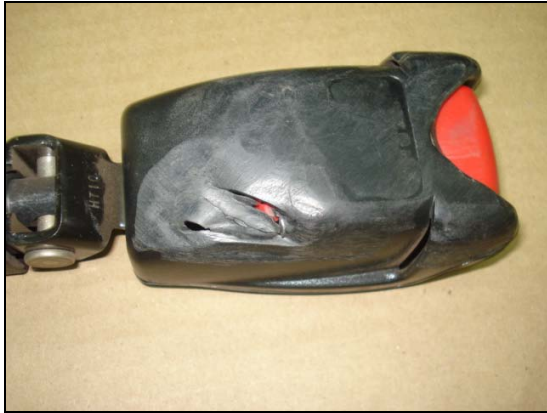
Wear due to abrasion or rubbing contact with buckle
