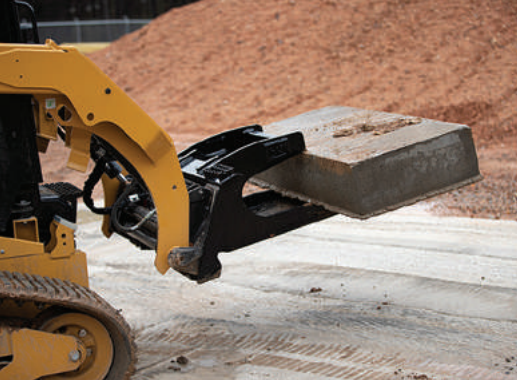
Concrete Slab Bucket
